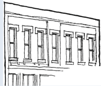
Existing building with missing cornice.
