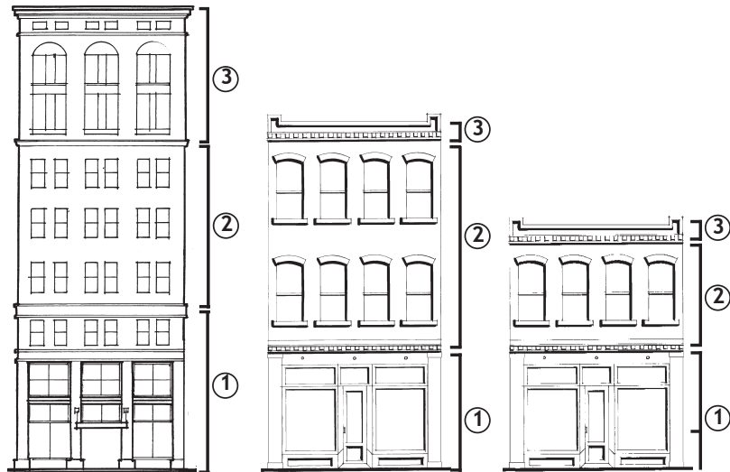
These three commercial buildings in a historic district, although of different heights and periods of design, share these elements: 1. Base, 2. Middle, and 3. Cap.
