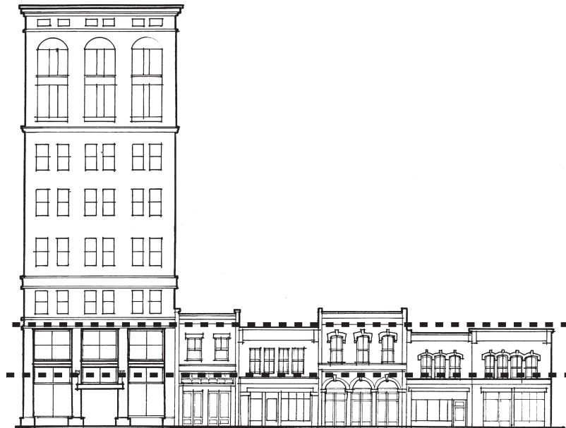
In many commercial districts, similarity of floor heights at the street level, and horizontal moldings combine to create a horizontal alignment that establishes a distinctive scale for a block, which is a character-defining feature.
